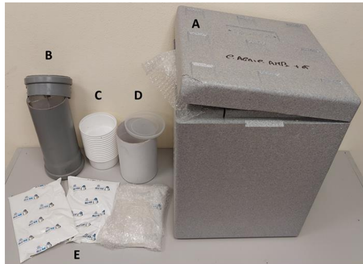
Fig. 1 – A) Polystystrene container; B) emerging tube (max. 2200 pupae); C) plastic cups for the adults; D) cardboard cylinder to hold cups; E) PCM gel packs (Blue Ice and Green Ice to maintain cooling during the transport of Aedes albopictus males.
