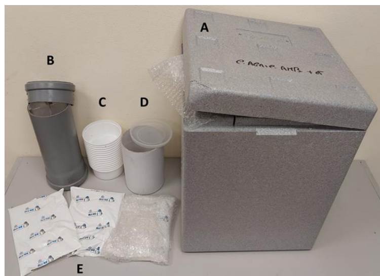
Fig. 1 – A) Polystyrene container; B) emerging tube (max. 2200 pupae); C) plastic cups for the adults; D) cardboard cylinder to hold cups; E) PCM gel packs (Blue Ice and Green Ice to maintain cooling during the transport of Aedes albopictus males).
